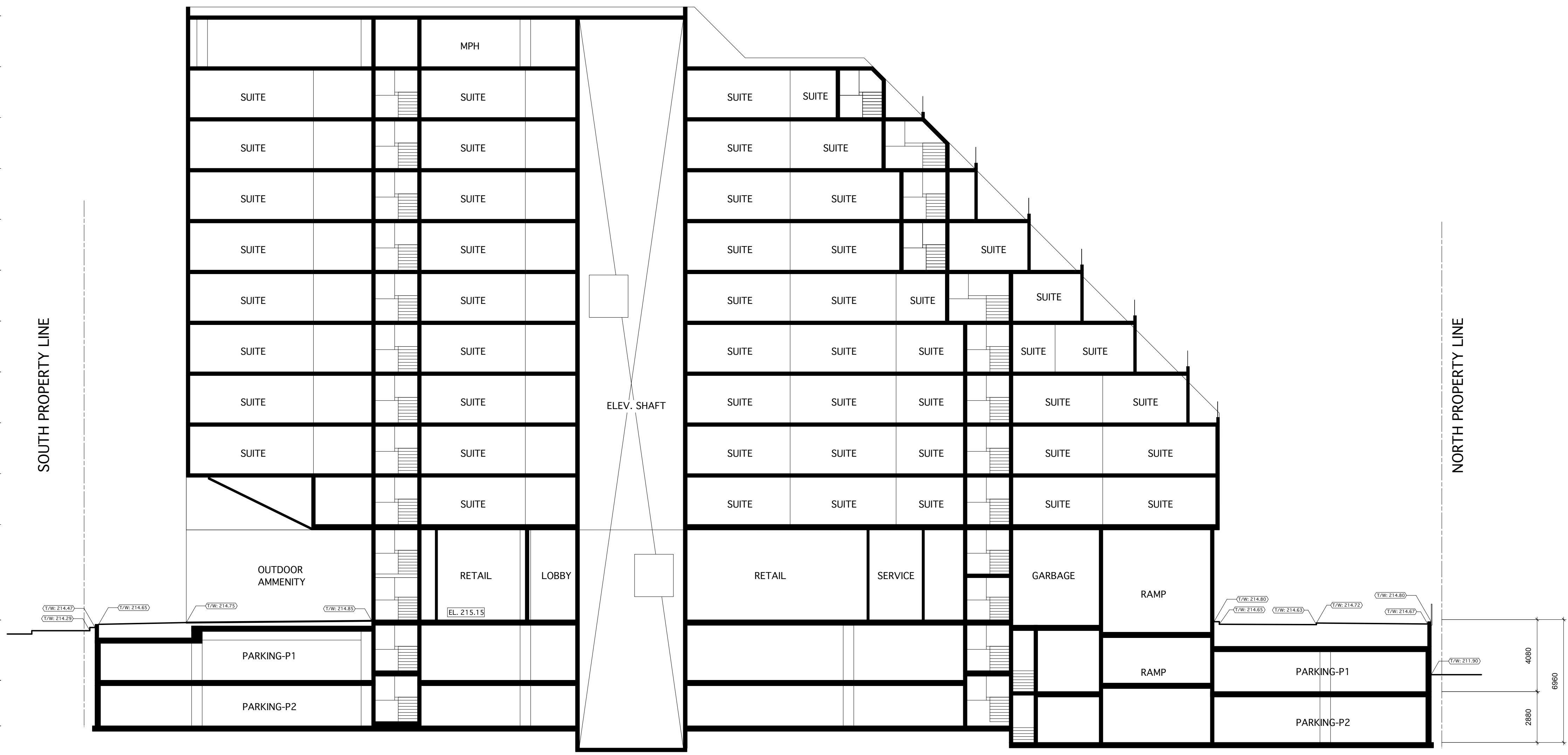
1 SP-4.1 BUILDING SECTION - NORTH SOUTH Scale: 1:150
